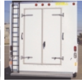
5 50" swing out doors shown with optional ladder rack and removable rear step ladder
