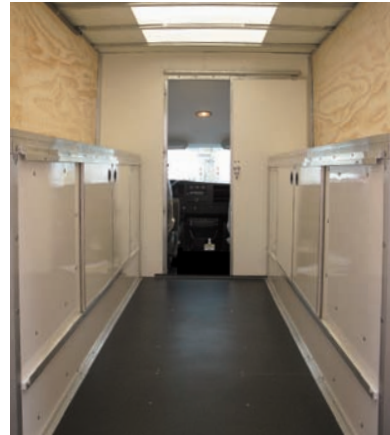
Shown with optional plywood lining and Unifloor
