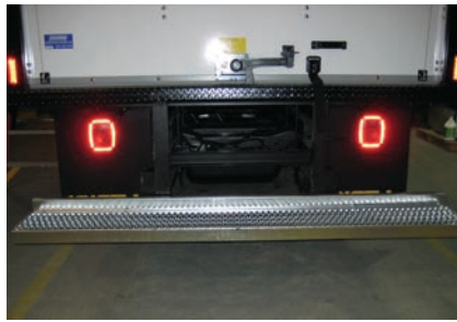
Full width galvanized steel safety-grip step bumper
