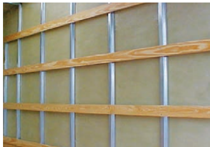
Standard slatted lining for optimal cargo retention
